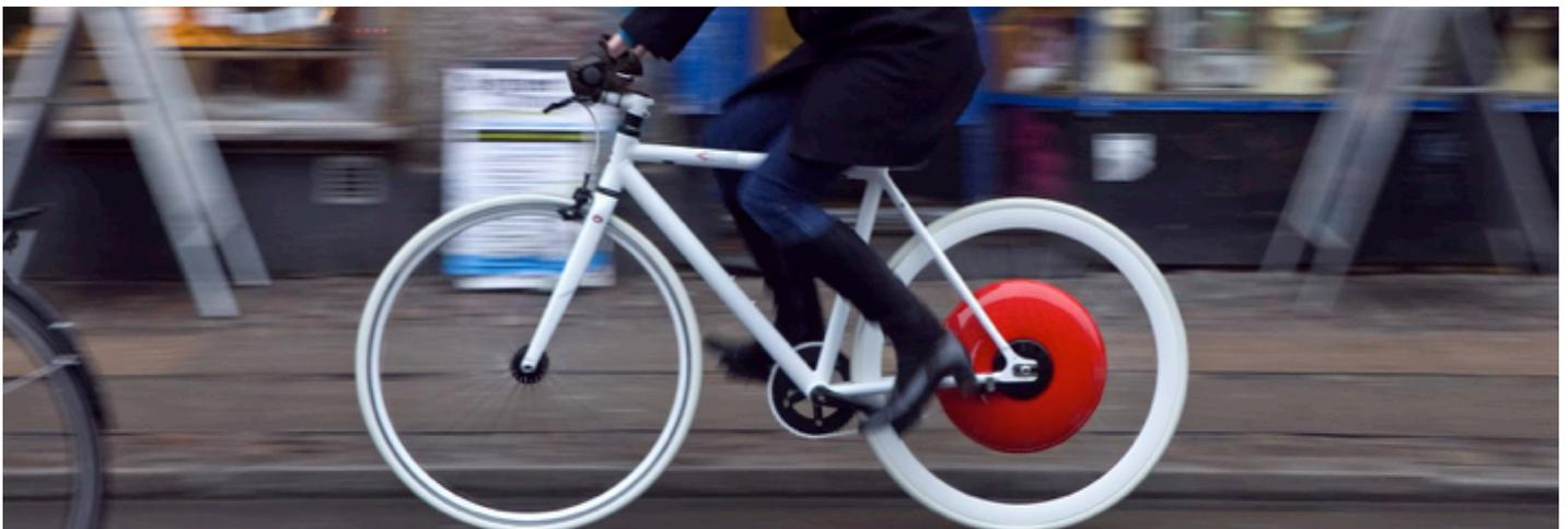
**Picture 4.** The Copenhagen Wheel transforms your bicycle into a smart electric hybrid. The Wheel contains a motor, batteries, multiple sensors, wireless connectivity and an embedded control system. The Wheel learns how you pedal and integrates seamlessly with your motion, multiplying your pedal power.
